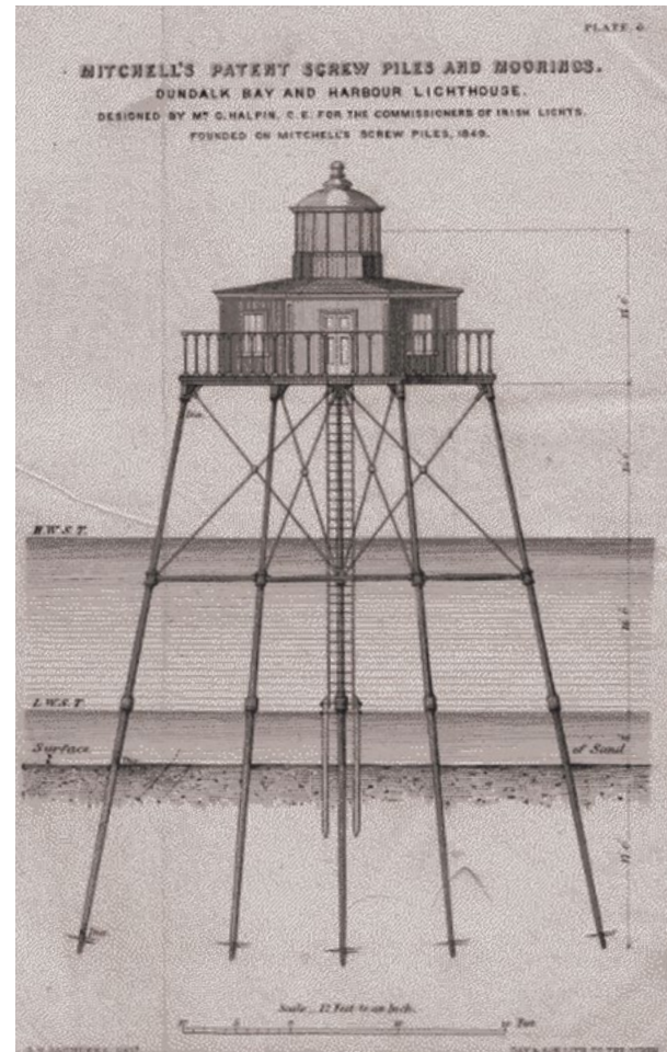
Figure 1.2 Early patent of screw (helical) piles
