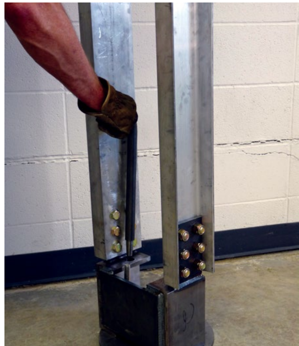
Figure 2.55 PP288 drive stand mounted to slab pier drive adaptor
