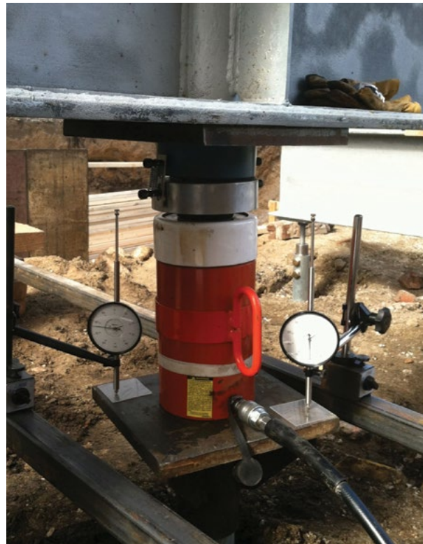
Figure 1.61 Close up of test pile, hydraulic cylinder, dial gauges and hemispherical bearing plate
