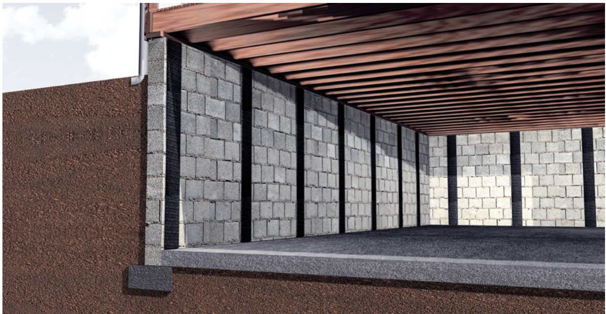
Rendering of the CarbonArmor® system installed within a basement
