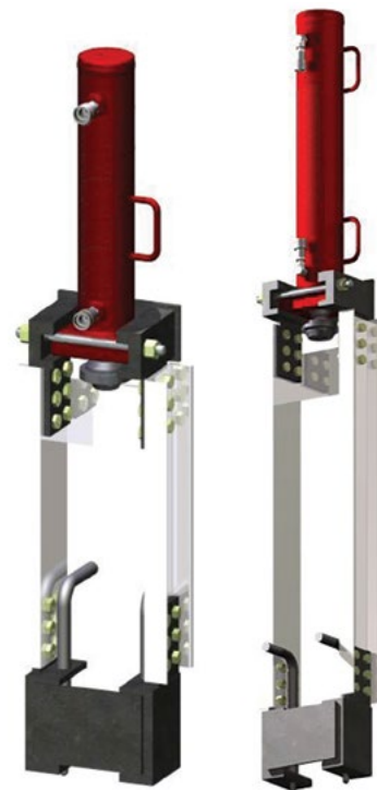
Figure 2.17 Crawl space and standard drive stand assemblies for the PP288 push pier system
