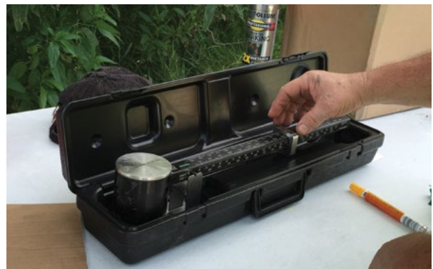
Figure 1.99 Measuring the specific gravity of the grout with a mud balance
