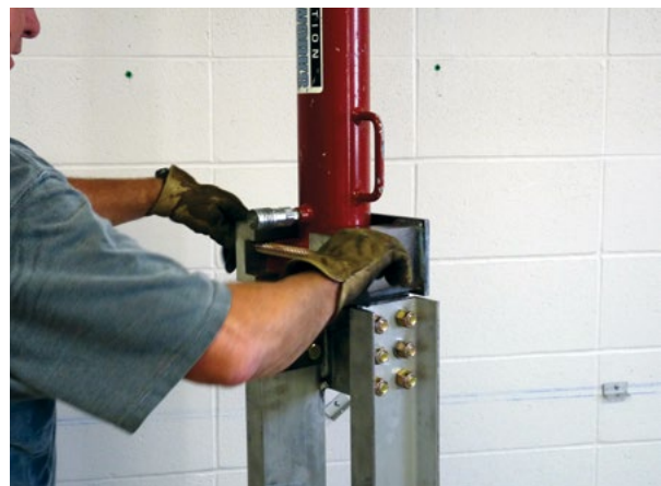
Figure 2.56 Drive cylinder set into top fixture of drive stand
