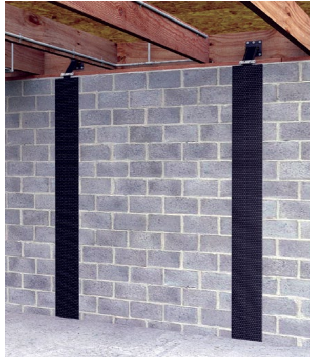
Figure 3.30 Rendering of CarbonArmor® installation with optional ArmorLock® connection to rim joist
