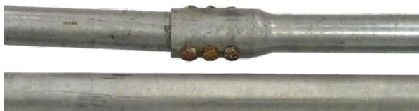
Figure 1.15 Competitor upset coupler variance from straightness
