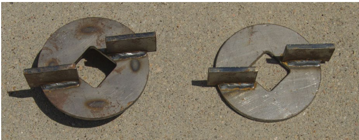
Figure 1.54 Lead displacement plates (cased on left, plain on right)
