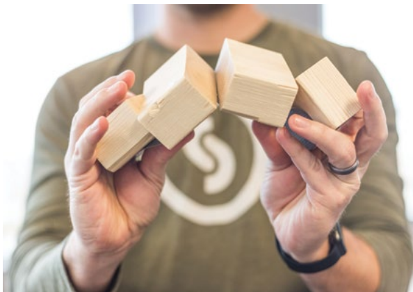
Figure 3.3 Stack of wooden blocks fan apart when bending force is applied
