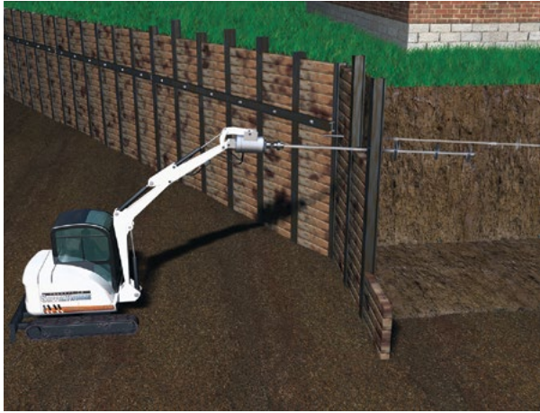
Figure 1.41 Rendering of helical tieback installation for soldier pile and timber lagging wall
