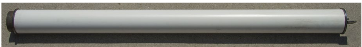
Figure 1.56 PVC casing between lead and first extension displacement plates
