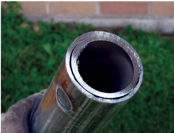
Figure 2.53 Starter tube made by cutting coupler end of standard pier tube
