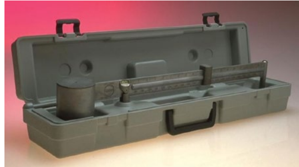
Figure 1.57 Mud balance for specific gravity testing of the grout mixture
